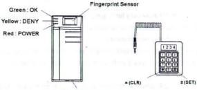
Hole to insert external keypad.
