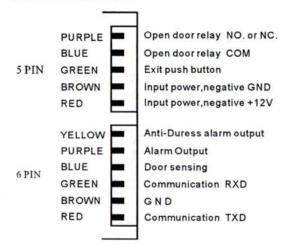
2. Wiring connection for additional electric lock and push button door open switch.
